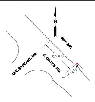
GPS 246, 2" BRASS DISK STAMPED 246, LOCATED ON INLET TOP ON E. OATES RD. APPROX. 53' SE OF E. OATES RD & CHESAPEAKE DR. INT. & APPROX. 24' NE OF E. OATES RD. C/L.
